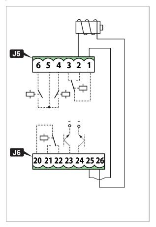
Connection of a magnetic lock that needs power to be removed in order to be released:
