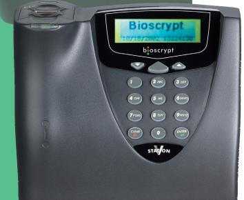
V-Station incorporates advanced fingerprint technology in a self-contained terminal. The V-Station can support both standard and proprietary Wiegand communication formats and stores up to 3000 templates on the unit. With an optional integrated proximity or contactless smart card reader or the 1–to–200 searching capability, the V-Station is the most flexible biometric solution available today.
